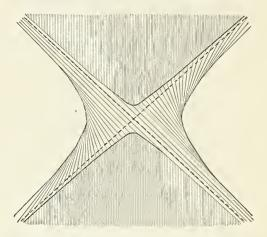
axis is vertical. By moving the cutting plane a little closer to the centre, the bounding curves of the section will merge into the dotted lines, and the plane will be a tangent to the surface at their point of intersection.
